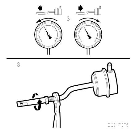
Rotating the end piece 1 turn changes the basic charging pressure by about 0.02 bar.
